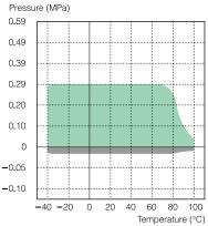
Working range applicable when combined displacement is 50% or lower.
